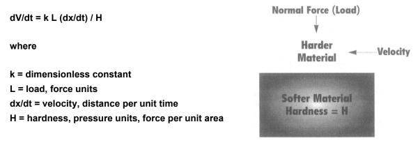
Figure 1. Basic components of a system undergoing abrasion.
