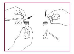
**Figure 4 –** A notched swab handle simplifies separating the swab head from the handle. Only the head needs to be extracted for TOC measurement.
